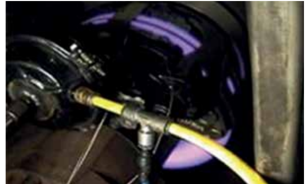
Brakes under high demand utilization reach temperatures over 500°C.
